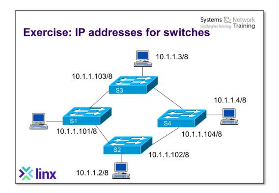
6. We will now give the switch an IP address. With end devices, IP addresses are configured on the network card. Switches can be seen to have 12, 24 or more network "cards", but the switch only needs one IP address. The address will be placed on Vlan 1 and can by default be accessed through any of the Ethernet ports on the switch.
